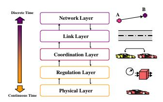
Figure 3. PATH Control Architecture.
