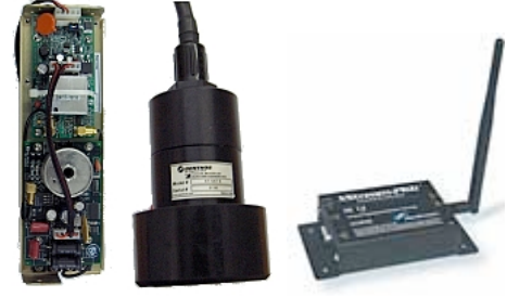
Fig. 1. Hardware: Benthos Acoustic modem (left) and transducer (middle) [3] (left) and MaxStream RF modem [3] (right).
