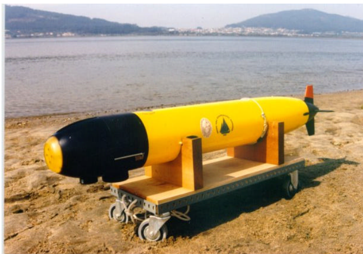
Figure 1 – The Isurus AUV
